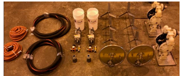
QPDS Parts (hoses, motors, regulator, mixing paddles, & polypropylene diaphragm pumps)
