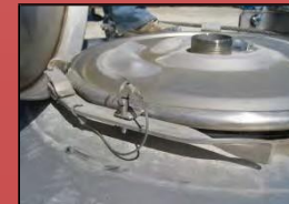
Quick-release-lever hold down ring NO TOOLS REQUIRED
