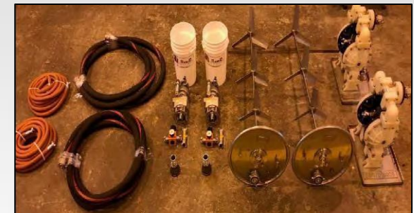
QPDS Parts (hoses, motors, regulator, mixing paddles & polypropylene diaphragm) pumps
