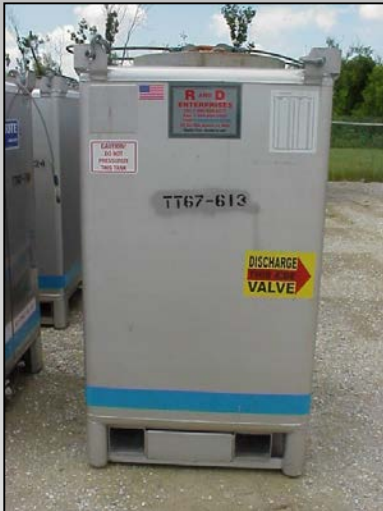
Bottom Ends Blocked to Prevent Oversized Forklift Damage
